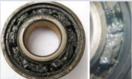
Competitor high contamination seal (after 32 hours)
