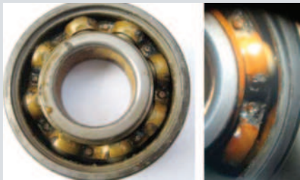
Typical standard seal (after 32 hours)
