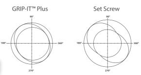
GRIP-IT™ Plus provides a greater than 50% improvement in raceway concentricity than a set screw lock after mounting.
