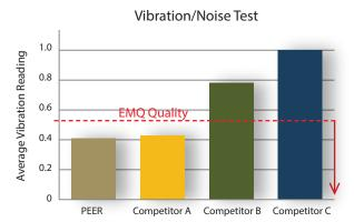
The data represents average vibration readings recorded during testing. This dimensionless value identifies the le el of vibration on a scale of 0–5, where zero is the lowest vibration level and 5 is the highest vibration level. Bearings with values less than 0.50 are considered electric motor quality.
