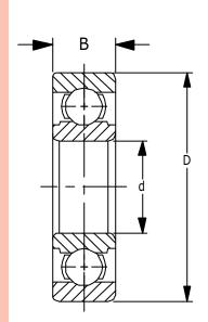
The 600 extra small metric series is produced in bore sizes ranging from 4mm to 9mm. These bearings are designed to take adequate radial and thrust loads in proportion to small shaft sizes. This series may be ordered open, shielded, with contact seals, or non-contact seals. Stainless steel 440C, 600 Series bearings are available upon request.
